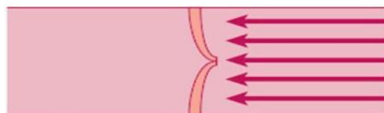
Valve closed; does not open in opposite direction
