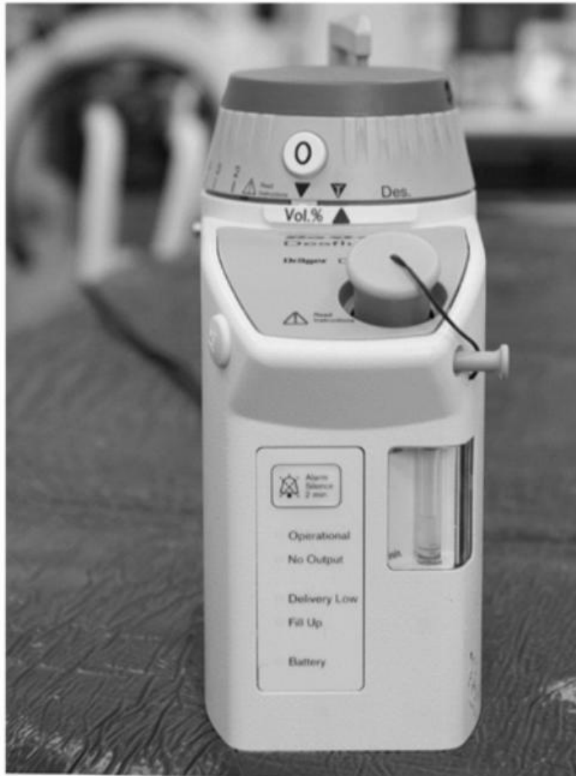
FIGURE 15.8 ■ Tec 6 desflurane vaporizer.
