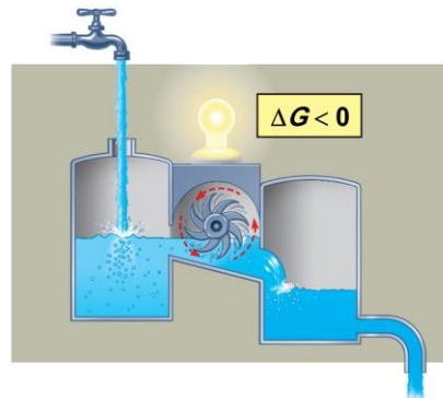
(b) An open hydroelectric system
