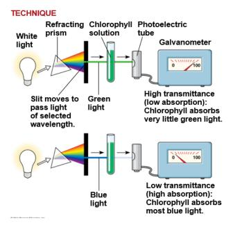
The ability of a pigment to absorb various wavelengths of light can be measured with an instrument called *"spectrophotometer"*.
